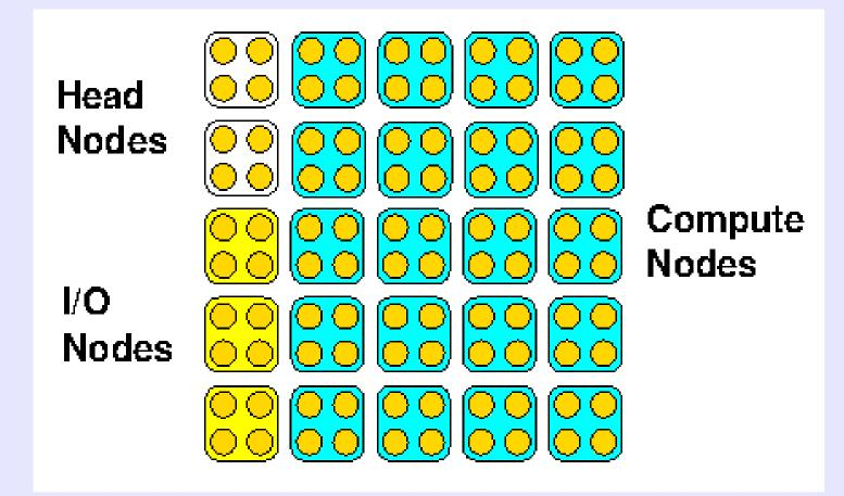
On typical cluster, the work must be done on the compute nodes. We could submit multiple single node job scripts, but how about using more than one node at a time?
